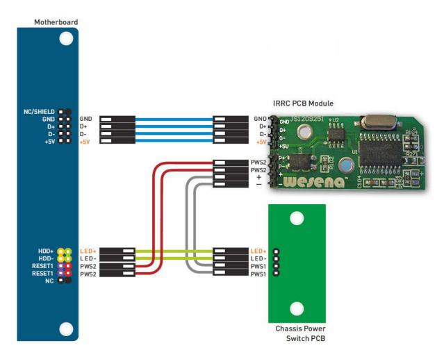
If the wires supplied with your IR Receiver are white, you will find that each wire has a different pattern running the length of the wire so you can use these patterns to ensure that you connect the correct the pins/components together.
