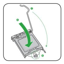
Insert the load lever under the retention tab.
