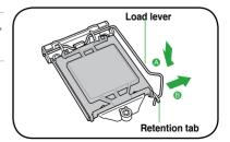
Lift the load lever in the direction of the arrow until the load plate is completely lifted.
