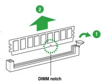
2 Remove the DIMM from the socket
