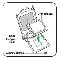
Close the load plate (A), and then push down the load lever (C), ensuring that the front edge of the load plate slides under the retention knob (B).
