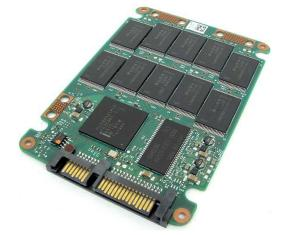
It's quite simple, really – MLC stands for *multi-level cell*, whereas SLC stands for *single-level cell*. This means that each *transistor* (or *cell*) in an MLC drive holds two bits of information, whereas in an SLC they only hold one.
